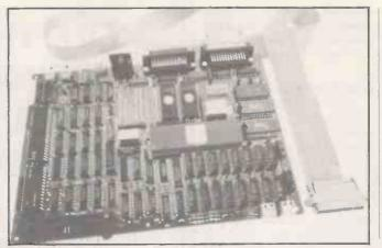
The Profi Kit 2 is a 16-bit single-board computer using the Motoroala 68000 processor. Designed by Force in Germany, the board is an upgrade of the Profi Kit 1. It includes 128K of RAM and serial, parallel and cassette ports. Profi Kit 2 costs £499 plus VAT. **Contact Microsystem** Services, PO Box 37, Lincoln Road, Cressex Industrial Estate, High Wycombe, Buckinghamshire HP12 3XJ. Telephone: (0494) 41661.
